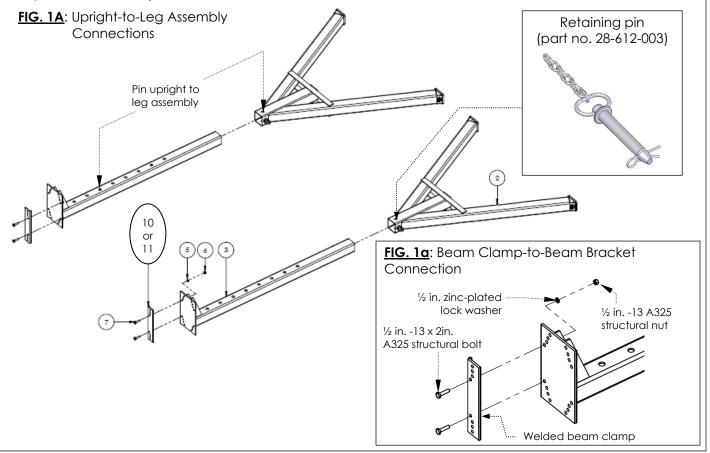
**Step 1B:** [Models AHS-6-20-12, AHS-6-20-14, AHS-6-20-16, AHS-8-20-12, AHS-8-20-14 & AHS-8-2016] Fasten the uprights to the leg assemblies; then fasten two beam clamps to the beam bracket.
