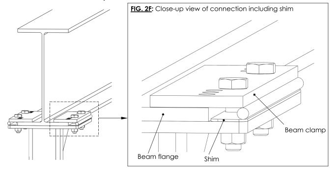
**Step 3:** Tighten the beam clamp fasteners to 50 - 52 ft 1b of torque.
